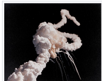
Challenger's solid rocket boosters fly uncontrollably after the breakup of the external tank separated them from the shuttle stack. The remains of the orbiter and tank leave thin white contrails as they fall toward the Atlantic Ocean.
